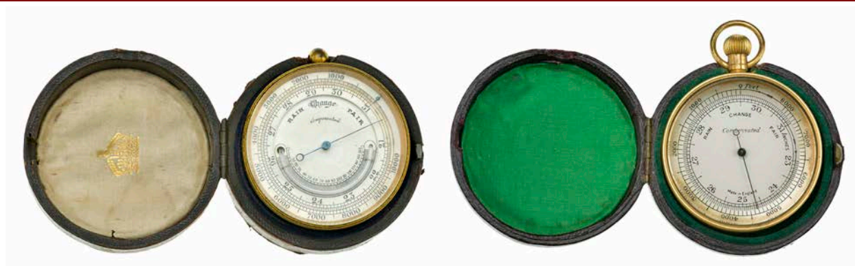
A GILT BRASS POCKET COMPENSATED BAROMETER, WITH ALTIMETER AND THERMOMETER , the dial with curved thermometer and 0-160 degrees Fahrenheit scale above, barometric scale of 21 to 31 inches, and revolving altitude scale of 0 to 8000 feet, blued steel hand, dial unsigned, in fitted case, the silk to the inside lid with gilt crown detail, together with a second gilt brass pocket barometer altimeter compensated science weather gauge, with rotating outer dial for altitude function, scale from 0 to 8000 feet, barometric sale from 23 to 31 inches, blued steel hand, with case (possibly unassociated case), first diameter 5cm, second 4.8cm. £100-200
